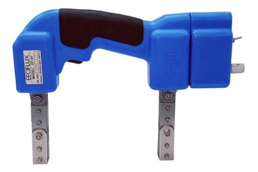
EF-9Y is a new generation electromagnetic yoke which can create AC & HWDC magnetic fields for detection of surface & sub-surface cracks during magnetic particle inspection.
